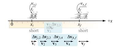
$$v_{x,i} + a_{x,AVG} \Delta t = v_{x,f}$$
